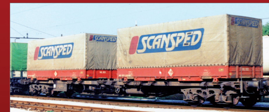
Carro Sgns danese caricato con due casse mobili telonate "SCANSPED". DSB Sgns container vogn belæsset med to "SCANSPED" veksellad. Danish type Sgns container wagon loaded with two "SCANSPED" swap bodies.
