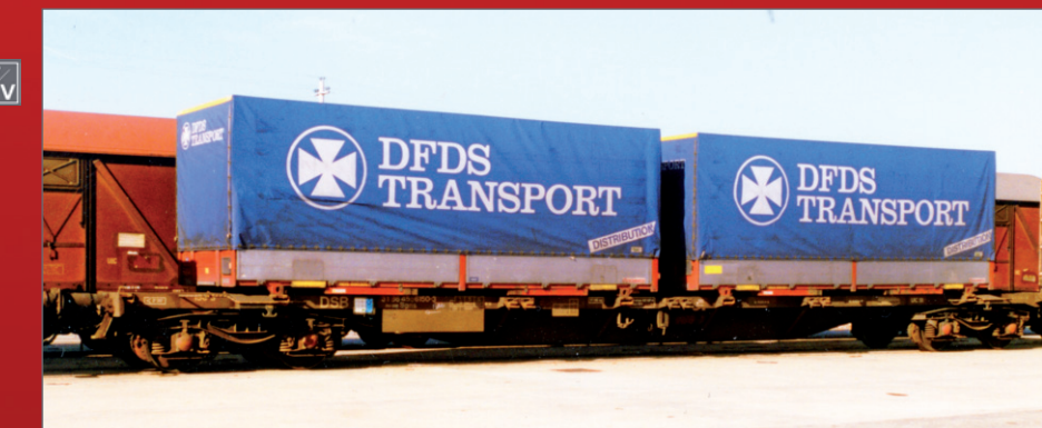
Carro Sgns danese caricato con due casse mobili telonate "DFDS TRANSPORT". DSB Sgns container vogn belæsset med to "DFDS TRANSPORT" veksellad. Danish type Sgns container wagon loaded with two "DFDS TRANSPORT" swap bodies.
